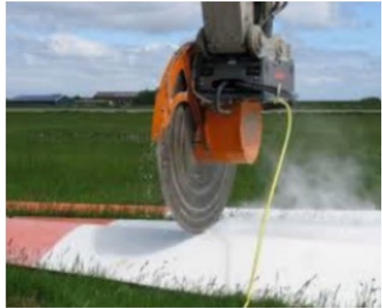
Figure 25 | Wind turbine blade cutting
